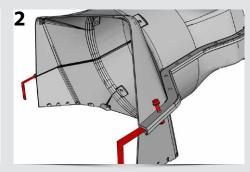
Place the side supports in position and mount the first bolt. The side supports are in between the upper and down part
