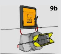
Mount the Air-Optimizer in front of a Flash 3300 inlet, this way you can adjust the ammount of fresh air vs the ammount of recirculation air.
