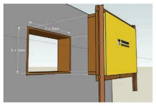
The Flash BP is made of high quality plywood and is available in many sizes. The hole in the wall should be 5 mm bigger.
